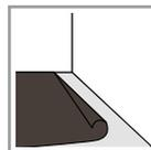
2. The installed boards must be provided with a covering or polyethylene sheeting without delay in order to avoid one-sided drying out.
