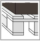
Before installation, the floor panel must be stored several days protected from water at the place of installation to allow it to adjust to ambient air conditions. The room temperature should be above 10 °C.
