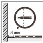
1. For the avoidance of creaking noises, an expansion gap of 15 mm should be left between the wall and the flooring board. The tongues should be removed for the first row. Intermediate expansion joints are required in the case of larger areas (more than 10 m in length).
