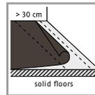
2. On solid floors in old and new buildings we recommend the use of vapour barriers made, for example, of 0.2 mm thick polyethylene sheeting. It should be laid with generous overlaps (at least 30 cm) or welded joints.
