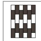
4. The boards should be installed in a bond with offset joints (offset by at least 15 cm) – i.e. without cross joints.
