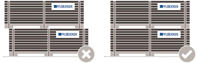
Wood-based materials react to changes of air moisture content and temperature, with equilibrium moisture content of panels changing in relation to the ambient humidity. Changes in panel moisture content lead to dimensional changes (shrinking, swelling).
