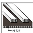
If vapour-tight sheeting is recommended to protect against moisture, a vapour barrier consisting of 0.2 mm thick polyethylene sheeting is used only on the underside of the timber beam floor (warm side), i.e. above the ceiling.
