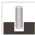
To ensure uniform glue application, please make sure that the dowel hole is up to 0.2 mm larger than the dowel. The use of rifled dowels is recommended.
