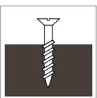
Predrilling is recommended with the drilling diameter equalling the core diameter of the screw thread. Screws should be positioned with a minimum distance of 20 mm to the panel edge.
