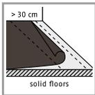
1. On solid floors in old and new buildings we recommend the use of vapour barriers made, for example, of 0.2 mm thick polyethylene sheeting. It should be laid with generous overlaps (at least 30 cm) or welded joints.
