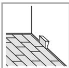
1. After installing all boards and before the glue has set, the boards should be wedged against the wall – for an optimum bond and to prevent creaking noises.
