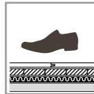
4. Better impact sound insulation is achieved by the use of mineral insulating materials. Glass wool insulating materials are recommended. In the case of higher requirements for impact sound, please use commercially available spring rail systems for sound insulation.
