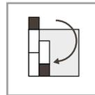
2. The remainder of the last flooring board of the first row can be used as the starting element of the second row in order to avoid wastage.
