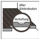
3. Depressions in the existing floors should be filled with loose, rot-proof bulk materials (e.g. natural expanded shale). Please do not use sand under any circumstances!
