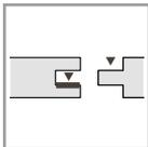
3. Apply white synthetic resin glue (PVAc) to the lower flank of the groove and the upper side of the tongue. Insert the flooring board with the tongue into the groove of the already installed area.
