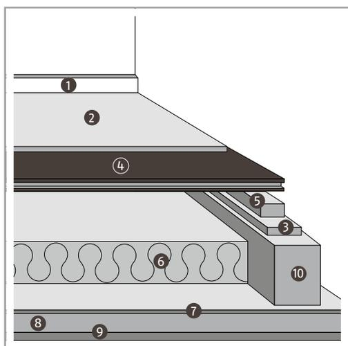
With renovations or even new buildings, building situations sometimes occur in which a board-type material of the type class P4 or higher must be installed on floor beams. We recommend the following procedure: A check should be carried out to ascertain whether thermal or moisture protection is necessary. Timber beam floors should not be covered on both sides with vapour-tight sheeting. The installation of insulating felt between the floor beams offers better thermal and sound insulation.
