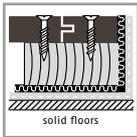
3. When screwing, care must be taken that the screws do not reach the solid floor. All insulations at the wall should be extended up to the top surface of the covering (approx. 10 cm), and the sheeting should remain intact – also during subsequent work. The overlap of the sheeting should ideally be located under the flooring sleepers.
