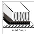
2. The height is adjusted by the use of different underlay material. Solid wood, hard fibre, plastic or raw chip board strips should be laid out for this. These are held together by wood glue when assembling.
