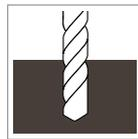
Proven and standard tools and materials for drilling plywood and solid wood must be used. For DecoBoard, boreholes should be lowered to avoid splitting.
