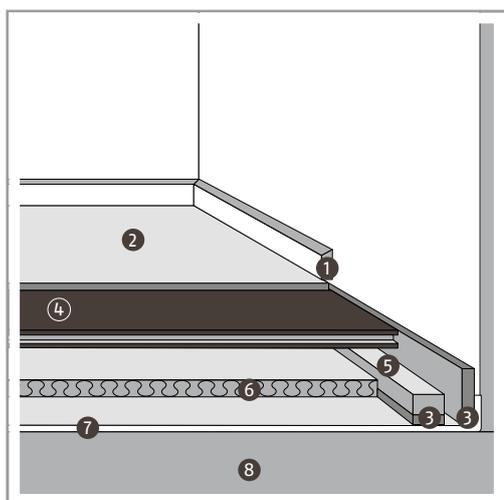
Flooring boards are frequently used in old buildings. However, since they often exhibit depressions several centimetres deep, they must first be levelled with bulk materials before the actual installation process. Installation on flooring sleepers is a more practical and cheaper alternative here. Boards of the type class P4 or higher must be used
