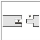
5. White synthetic resin glue (PVAC) should be applied to the lower flank of the groove and the upper side of the tongue. Gluing increases the overall rigidity of the board.
