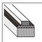
For reasons of sound insulation the flooring boards should not be installed directly on the timber beams. It is better to use a softly elastic covering and additional flooring sleepers here.
