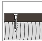
6. In accordance with the top covering the screws should be filled if necessary and possibly pre-drilled with a countersink bit. **Use screws with a full thread (not partial thread)!**
