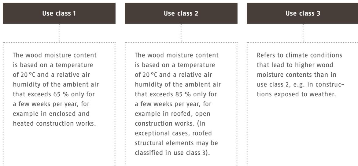
Sheet materials of use class 3 can also be used in use classes 2 and 1, high load-bearing panels are also used for load-bearing and non-loadbearing applications.
