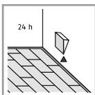
3. The wedges can be removed following an appropriate glue drying period (about 24 hours).
