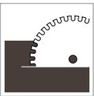
Due to their excellent quality, panels from Pfleiderer allow easy machining with all standard saw types. Tungsten carbide saw blades are recommended. For MDF finish cut grades and cut-to-size sheets, a cutting angle of 8 to 10 degrees and a cutting speed of 40 to 80 m/s are best to achieve optimum results.
