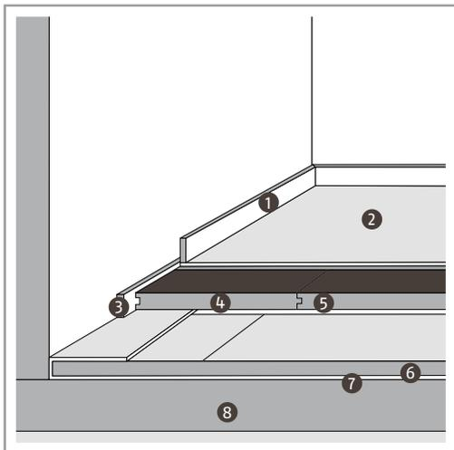
The most common type of laying tongued and grooved panels is the installation of floating floors described below. For normal loads the panel thickness should be at least 22 mm.
